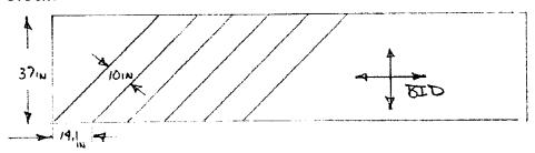
Prep the aft face of the center section spar stub "C" for a flox corner. Use tape to protect the <u>forward</u> half of both top and bottom faces of the spar core from epoxy slop while the aft shear web lay up is made. Mark the <u>aft</u> edge of the tape with a bold colored marker line down the length of the spar to aid in knife trimming the shear web lay up. Cut two 80 inch long strips of 4 inch dacron tape peel ply.
