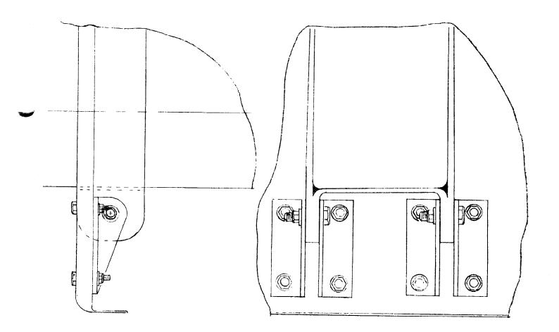
Before removing the wings, cut strips of .032 aluminum (6061-T4, 5052-H34, or 2024-T3) to make a wing root gap seal. Fit  $3/32 \times 3/8$  (aircraft spruce #2) rubber channel onto the inboard edge as shown in the sketch. The gap seal should be a tight fit to the fuselage side on both top and bottom surfaces. Pop rivet the seal strip each two inches as shown.
