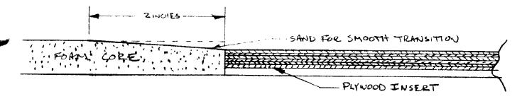
Mark the foam with positions of bulkheads, side consoles, instrument panel, wing cut-out, aileron pushrod and flap torque tube holes, wing chordline reference, and F.S. 53.0 reference lines. Sand the bottom edge corner blocks for a smooth transition into the flat side panel forward and aft of the wing/gear attach insert. Go cut the cloth and peel ply listed below:
