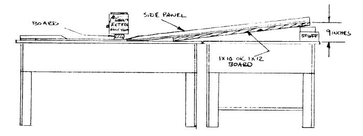
Curing the side panels in this fashion will aide in assembling the sides and bulkheads without needing the Green Bay Packer's defensive line to help out. Keep the long board parallel to the top edge but relatively centered in the width of the side panel's aft end.
