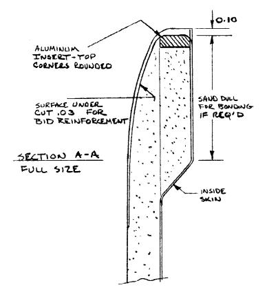
Next, use your rotary file to prepare a flox corner along the top edges from the firewall aft to the tail attach bulkhead. The canopy attachment inserts don't get a flox corner.
